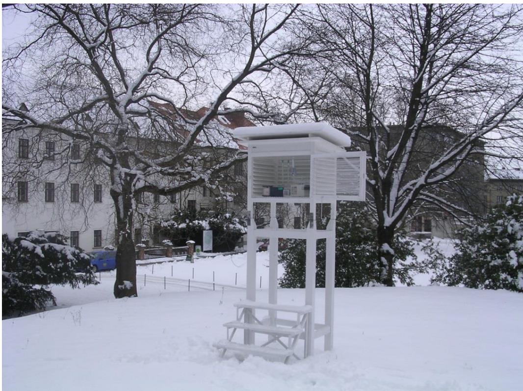
**Fig. 3** Stevenson screen with automated station including standard equipment for demonstration purposes
